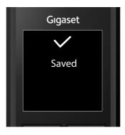
The display shows **Saved**. You will hear a confirmation tone and the handset automatically reverts to idle status, or returns to the "Settings" menu if the setting was made via the menu.
