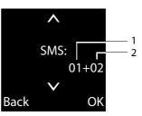
Open list with OK. An entry in the list is displayed with the number, status (old or new) and the date of receipt (example):
